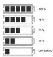
The display on the top half of the Illuminated LCD screen is the battery life indicator. This indicates the level of charge – more bars indicate more charge, while fewer bars mean less charge.
