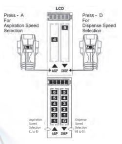
The user-selected speed will be stored in the internal memory so that, after being on standby, when the user starts working again, they can start with the previously selected speed.
