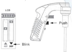
The user can decrease the dispensing speed electronically to its lowest level [G] during the dispensing operation by pressing the EBS™ control switch (08) for a precise stop at the desired volume. Check 3.1.9 EBS™ (Electronic Brake System) for more detail.
