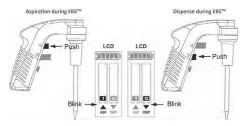
You can readjust the speed by pressing A/D on the Speed Selection Switch (09).
