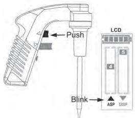
The user can decrease the aspiration speed electronically to its lowest level [1] during aspiration operation by pressing the  $EBS^{TM}$  control switch (08) for a precise stop at the desired volume. Check 3.1.9  $EBS^{TM}$  (Electronic Brake System) for more detail.
